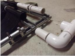
Clamp the edge bar (chain link fence top rail) to the 12" Unistrut using a #32 all 316 SS hose clamp. Two are shown in the photos above but only one is necessary.
