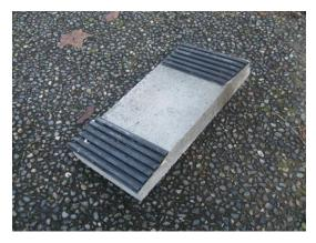
First lay out the ballast blocks. Its important they are 1.5" tall because this will orient the cross bars to be above the fin tubes precisely. If the roof surface is sensitive glue 7.5" long pieces of fin tubing under the ballasts as shown. Use Loctite Premium 3x PL (PL). Alternatively these pads can be placed under as the last step and because the ballasts never move they don't need to be glued.
