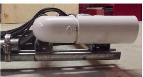
As you glue the manifolds to the 9-5/8" long intermediary pipes and couplings you may have to adjust the lengths of these intermediary pipes as necessary to line fin tubes up with each other.
