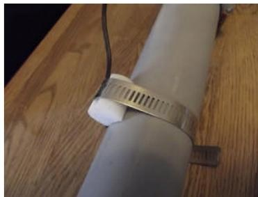
The "o ring" is a standard "dash 202" made of epdm or silicon. The band clamp is a #32 for 1.5" pipe or #40 for 2" pipe. The sensor head is machined for 2" or 1.5" nominal diameter pipes.
