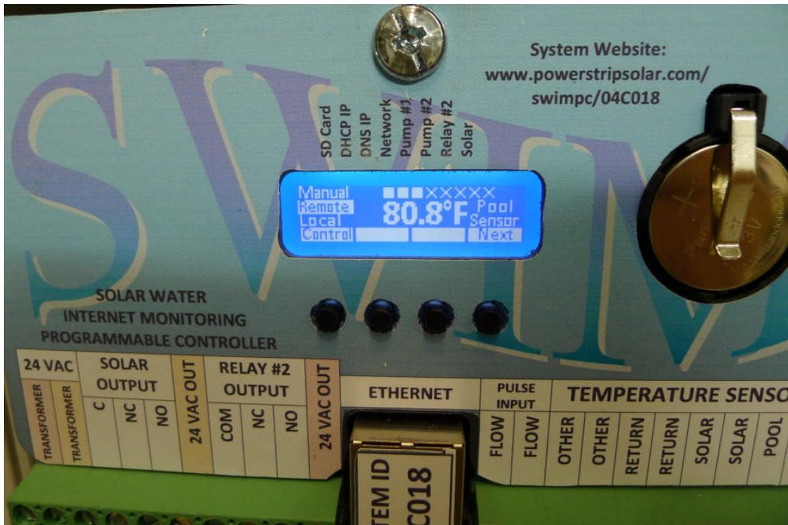
There are 8 indicator lights across the top of the display. X means off and square means on. In order left to right they are
